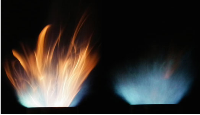
Fig. 23 Effect of droplet size on the flame color
